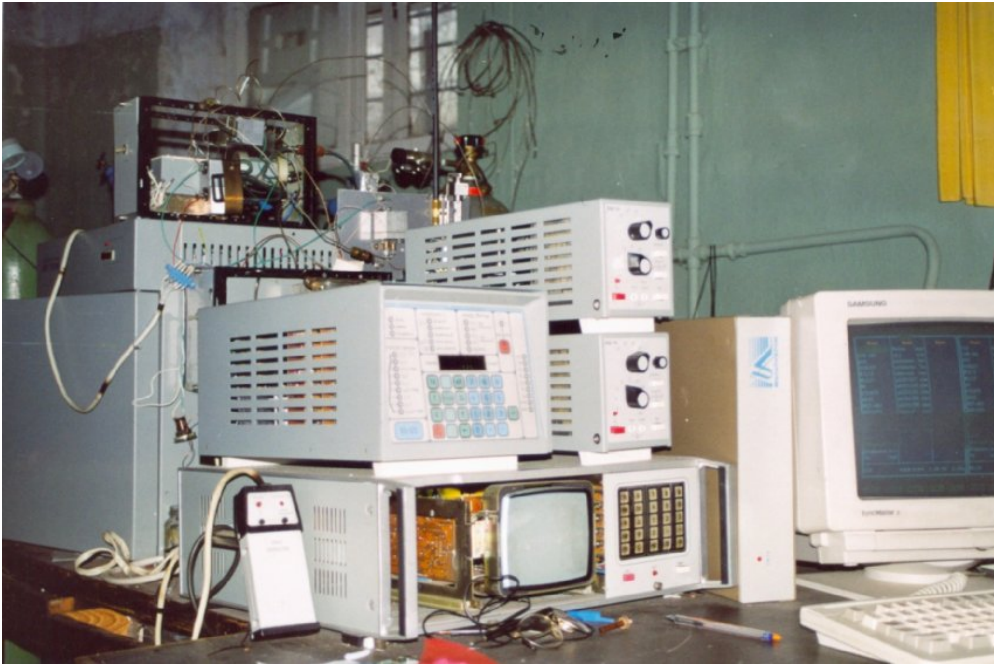
Fig. 3. An automated gas chromatograph (GC) system for CH 4 concentration measurements in the ambient air
